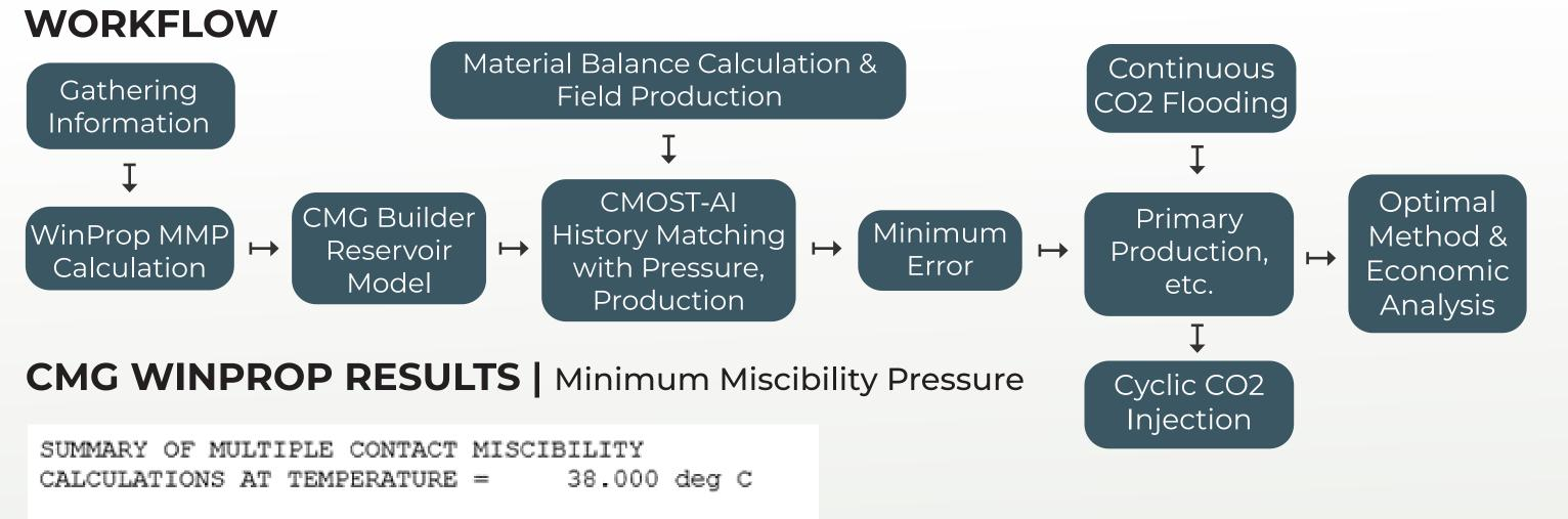
MULTIPLE CONTACT MISCIBILITY ACHIEVED AT PRESSURE = 0.95820E+04kPa MAKE UP GAS MOLE FRACTION = 0.00000E+00BY BACKWARD CONTACTS - CONDENSING GAS DRIVE
