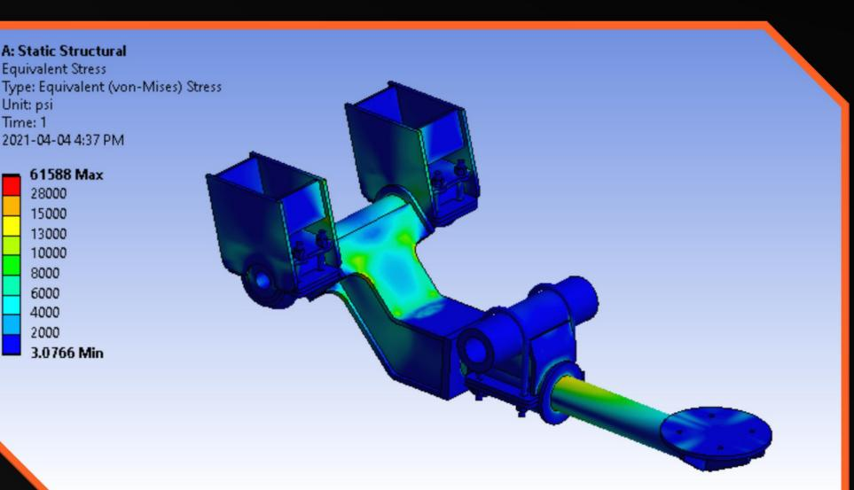
\*Stress riser due to inability to correctly model welds\*
