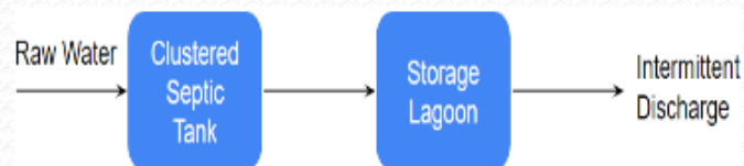
Figure 1: Process flow diagram for chosen design
